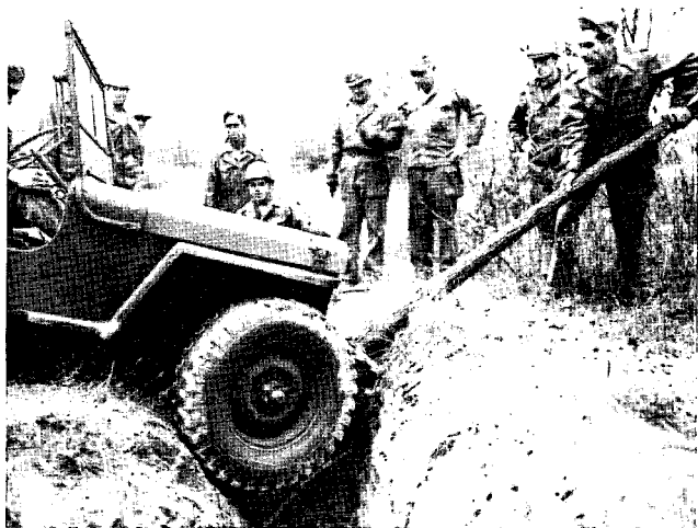
Figure 51. Pole used as a pry.
